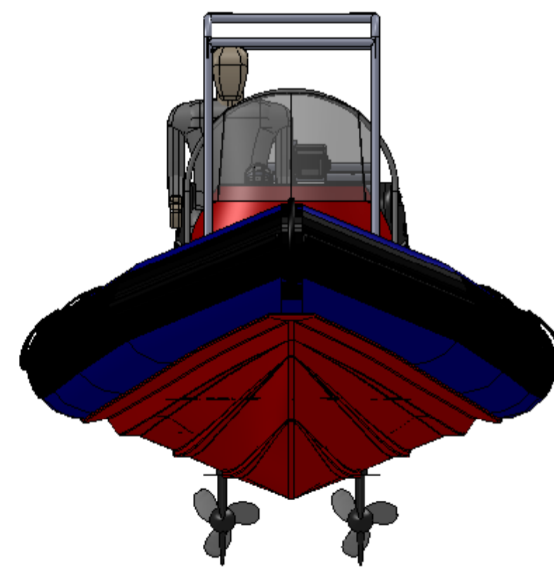
KEELGAURD RUNNING THE FULL LENGTH OF THE HULL
