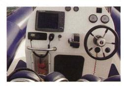
The consoles on these Offshore boats are set well forward providing an opportunity to mount a wide variety of seating options whilst still maintaining the balance of the craft. Options of console styles range from simple 'stand at the helm' commercial versions to wide curved creations with
